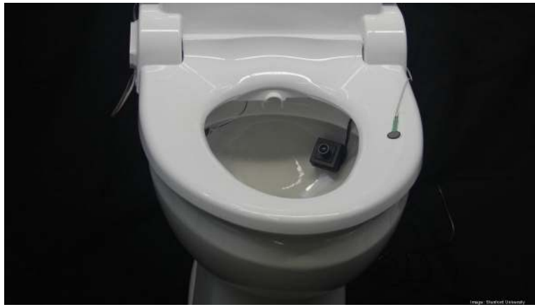
Figure 18. Stanford University Precision Health toilet with (i) Pressure sensor, (ii) Motion sensor, (iii) Urinalysis, (iv) Stool camera to monitor for CoViD or other health issues, (v) Anus camera to provide biometric identification, and (iv) Uriflow camera. Using AI and computer vision, the toilet performs medical diagnostics for early alerting of health issues. This is a good example that highlights the need to also consider priveillance which is the interplay between privacy, surveillance (being sensed) and sousveillance (self-sensing) as outlined in Section 13.1.
