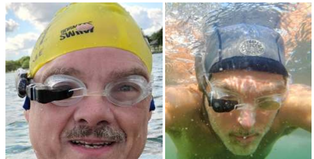
Figure 23. Vuzix Smart Swim underwater augmented reality system capable of displaying maps, wayfinding, etc., as well as live video feed from overhead drone for the SafeSwim [43] project.
