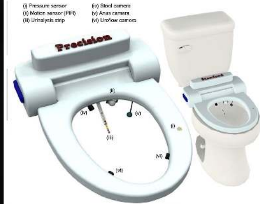
Figure 18. Stanford University Precision Health toilet with (i) Pressure sensor, (ii) Motion sensor, (iii) Urinalysis, (iv) Stool camera to monitor for CoViD or other health issues, (v) Anus camera to provide biometric identification, and (iv) Uriflow camera. Using AI and computer vision, the toilet performs medical diagnostics for early alerting of health issues. This is a good example that highlights the need to also consider priveillance which is the interplay between privacy, surveillance (being sensed) and sousveillance (self-sensing) as outlined in Section 13.1.
