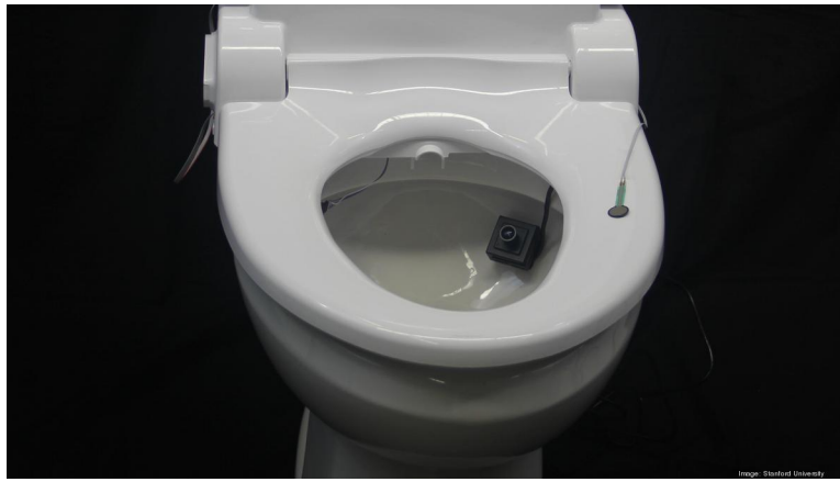
Figure 18. Stanford University Precision Health toilet with (i) Pressure sensor, (ii) Motion sensor, (iii) Urinalysis, (iv) Stool camera to monitor for CoViD or other health issues, (v) Anus camera to provide biometric identification, and (iv) Uroflow camera. Using AI and computer vision, the toilet performs medical diagnostics for early alerting of health issues. This is a good example that highlights the need to also consider priveillance which is the interplay between privacy, surveillance (being sensed) and sousveillance (self-sensing) as outlined in Section 13.1.
