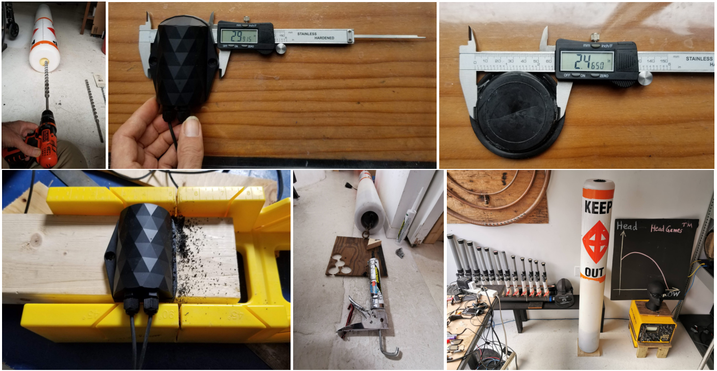
Figure 14. Building the Smart Buoy prototype. We first drilled out an existing buoy and then used cord seals having the computer and radio and antenna unit inside the hollow of the buoy and the sensor hanging down into the water. One lesson learned is that most buoys have only a very small opening, yet most sensing equipment is quite large. Here the sensor was almost 3 inches at its fattest point and would not fit through a standard 2.465 inch opening, so we had to trim it down while maintaining its waterproofness. (Bottom right) pictured at our lab with some of the other artefacts of our research: hydrophone, underwater oscilloscope, and chalkboard illustrating HeadGames™. (system for teaching hydraulic head as a function of flow.)
